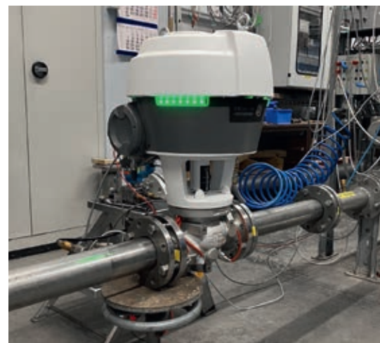
FOCUS-1 Smart process node for flow and decentralised process control
