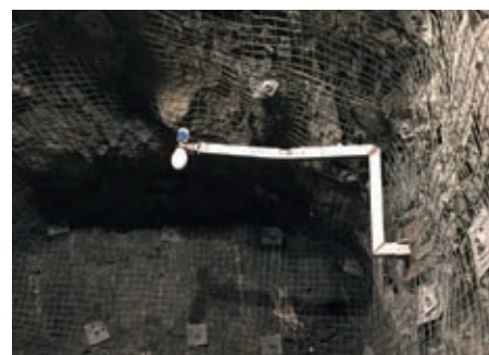
Level monitoring in an ore pass
