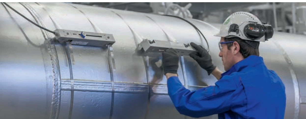
Clamp-on flow measurement on large line size
