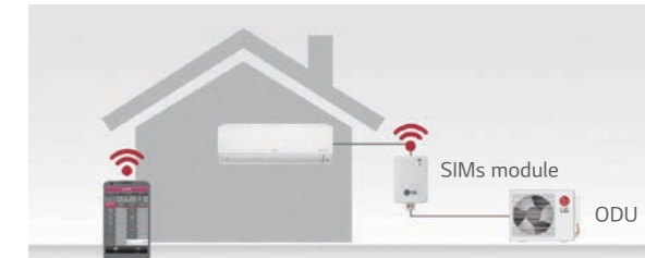
* SIMs : Smart Inverter Monitoring System
