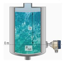
P<sub>hydr</sub> [bar] = hydrostatic pressure
