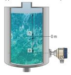
Zero point of the transmitter can be shifted up to the 50% of the range. Doing so the active measurement range will be reduced by the distance of "e"
