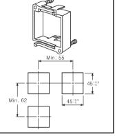
Using the optional **PAM-500-0** front panel adapter the 48x48mm sized unit can be mounted to an existing 96x48mm cut-out hole. In case of using the front panel adapter, the width of the mounting-plate is
