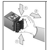
To select the input mode it is necessary to detach the housing. Before performing the operation always make sure that the device is powered OFF!
