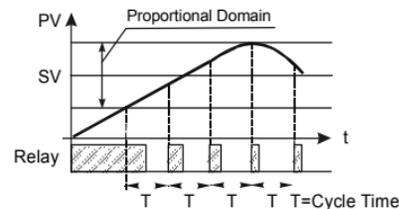
PID control with relay output
