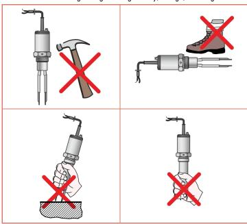
Before installation it is advised to try the operation of the level switch in a small sample of material in order to set the proper density. Tightening of the model with thread process connection should only be done with open end SW41, SW46 or SW55 spanner.
