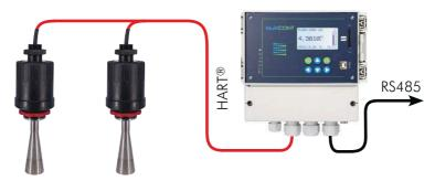
The MultiCONT can handle digital data coming from HART® capable NIVELCO transmitters (e.g. level, temperature, pressure, pH, dissolved oxygen, etc.). The digital (HART®) information is processed, displayed and transmitted via RS485 communication line to a PC when needed. Remote programming of the transmitters is also possible. Visualisation on PC can be accomplished with NIVISION process visualisation software.
